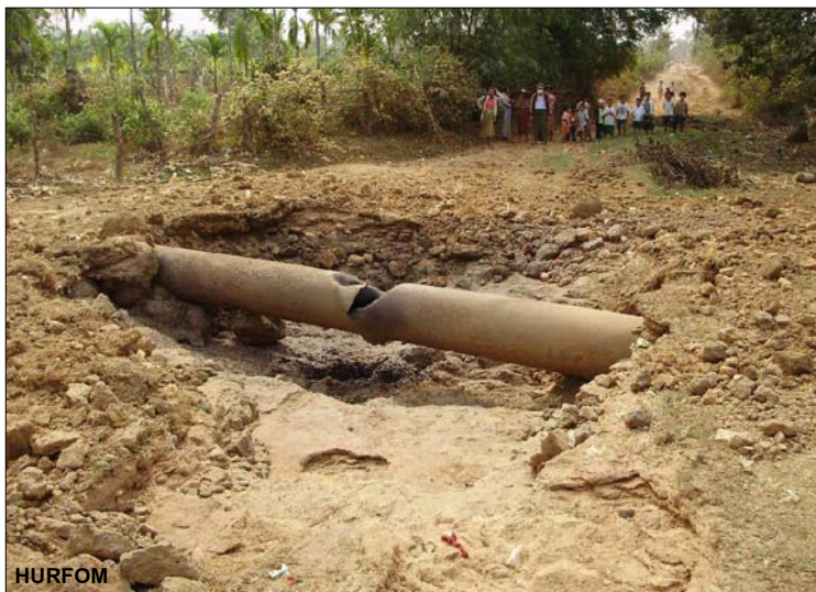
HURFOM Ruptured pipeline surrounded by a crater left by escaping gas near Lamine Town, northern Ye Township
