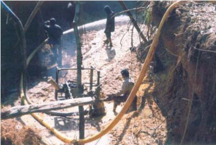
Water blasting to clear land for gold mining area in Tong mali; hydraulic mining in Nambyu
