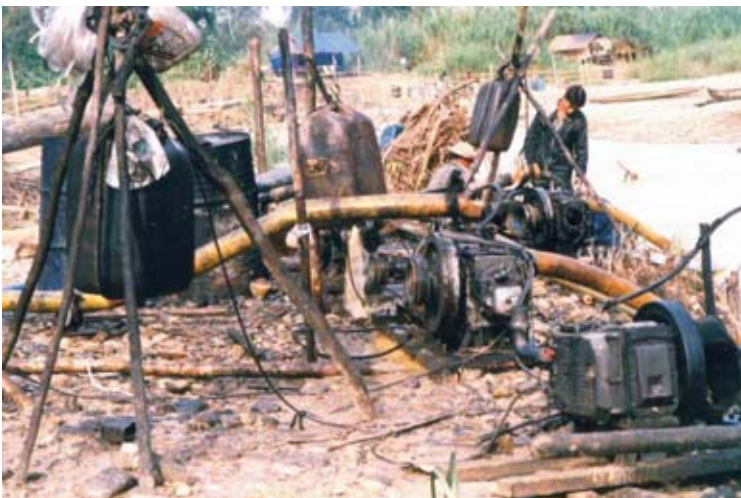
Diesel-powered pumps provide water to blast river banks for hydraulic mining
