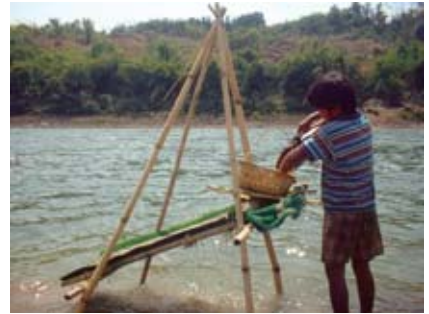
Workers pour earth through sieves in the Shingbwi Yang area after the land has been blasted away by hoses in the background
