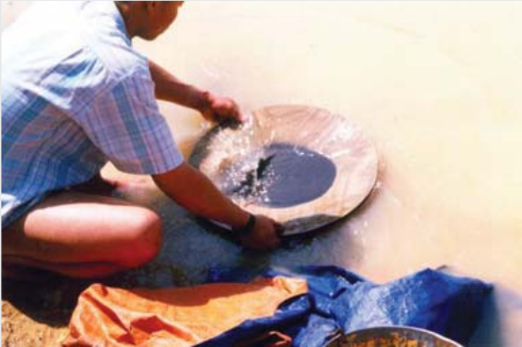
A miner pans for gold in the Nambyu area; using mercury to amalgamate the gold
